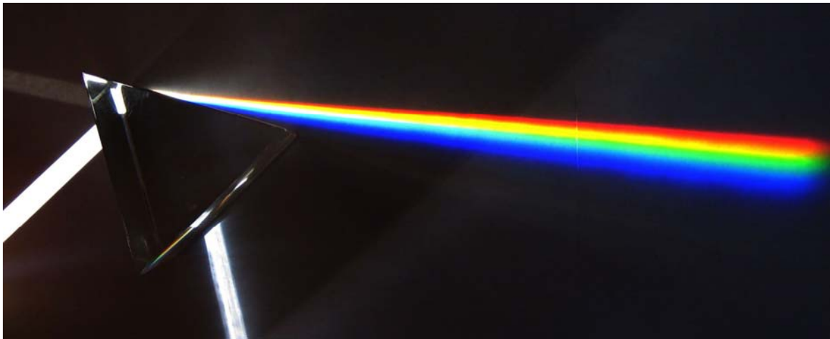
Fig. 7. Light passing through a transparent glass prism.
