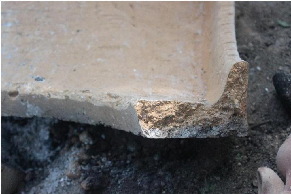
*Fig. 7. Partial burning of the clay*
