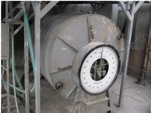
Fig. 2. *Ball mill*
