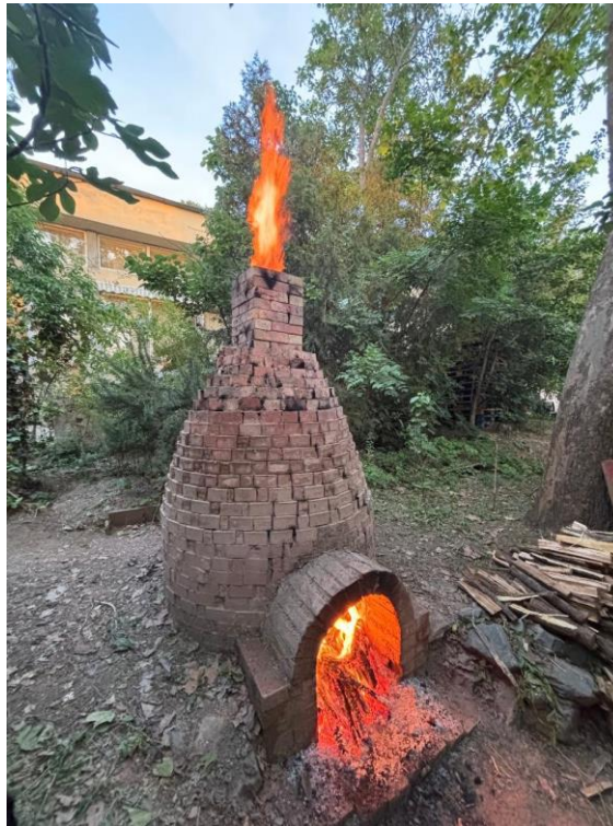
Fig. 1. Two-chamber brick oven with wood fuel
